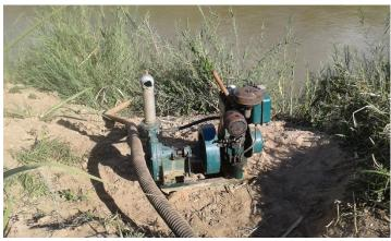
There are three schemes with mechanical pumps which are diesel or petrol driven. These have been problematic from the outset because there was no provision for the farmers to have fuel and no plan for ongoing maintenance. pumps are in poor condition or non-operational. With advances
